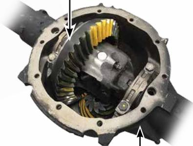
Powder-coated housing for maximum corrosion protection
