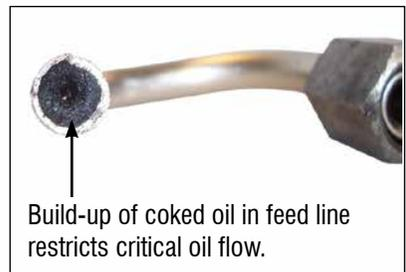
Upgraded oil feed line included to prevent failure, as a clogged line is the most common cause of failure for this application
